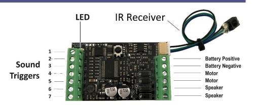
connections on the left trigger the various sounds where the locomotive controller has the appropriate outputs available. The trigger terminals are labelled F1 to F7 and are referred to by these labels in these instructions e.g. "Triggering F1" means to close a contact between the F1 terminal and the Battery negative terminal.
