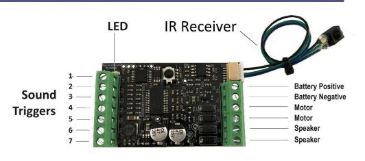
the left trigger the various sounds where the locomotive controller has the appropriate outputs available. The trigger terminals are labelled F1 to F7 and are referred to by these labels in these instructions. For example, "Triggering F1" means to close a contact between the F1 terminal and the Battery negative terminal.
