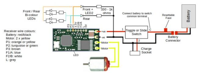
The default speed controller PWM frequency is 16kHz which works well for small and coreless motors. Larger motors may exhibit a reduced throttle response at this high frequency and will benefit from lowering to 1kHz or 500Hz - experience with Re280 type motors shows that 500Hz or 250Hz works best. The PWM frequency may be set using power-on programming changes or by programming MR601a, which requires a transmitter capable of programming receivers (e.g. Tx20, Tx22, Tx24 - not Tx10 or Tx21).
